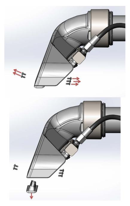
To replace the Glide, apply silicone sealant around the edge of the glide. Place the new Glide into the bottom of the wand head replace and hand tighten the five screws. If reattaching a glide that has already been used, lightly rotate the screws back and forth into the glide to find the original thread cut into the glide and hand tighten screws. Test the wand operation before returning to service.
