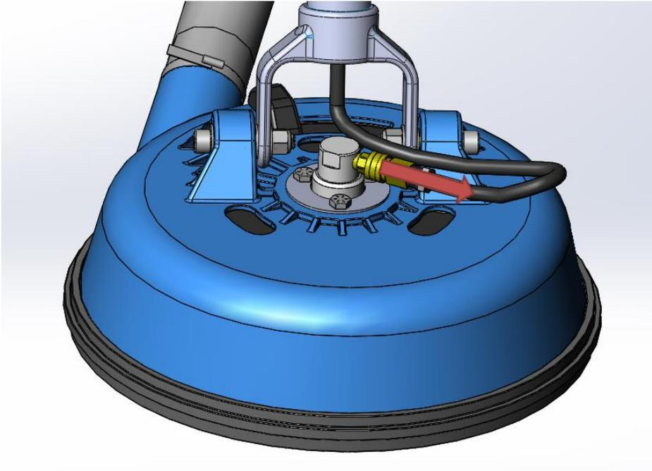
2. Remove the three assembly bolts at the base of the swivel
