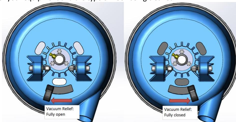
Using the SX-12 with extractors with higher air flow will generally require the vacuum relief vents to be opened more.
