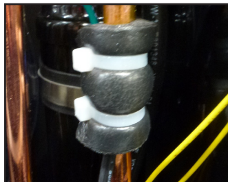
Figure 6: Thermistor attached to the refrigerant line.
