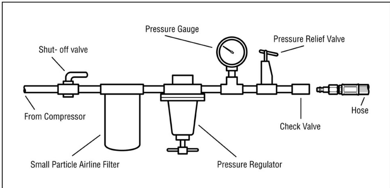
Oil mist from the compressor lubricating oil must not be present when the air reaches the air control device. Excessive amounts of water vapor and any particulate matter should also be removed as they may result in unpredictable behavior of the air control device. The schematic diagram (Fig. 1) of the air purifier and pressure regulator equipment shows what should be installed in the main airline ahead of the connection for breathing air hoses.
