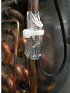
Thermistor attached to the refrigerant line.
