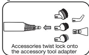
The accessory tool adaptor (#4 on parts overview page) is required when using the jet nozzle attachment, detail scraper, and all round detail brushes (#5-12 on parts overview page). Align the accessory with the arrow on the accessory tool adapter and twist to lock into place. The accessory tool adapter can be used directly on the steam gun or can be used with the extension tubes. (Fig.2 and 3)
