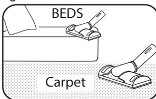
Apply light consistent pressure and slowly pass it along the surface (1" per second) to ensure the area being treated has a chance to come to full temperature, thereby killing pests and their eggs. (Fig.3)
