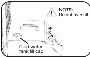
To fill the cold water tank, remove the rubber tank cap located on the top of the machine and using the supplied funnel, fill the tank (4.2 ltr / .80 gal). If filling without measuring, fill to the mid-level of the fill neck screen. (Fig.1)
