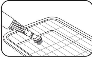
**⚠ IMPORTANT :** With all brushes it is important to not apply excessive pressure or force. This can cause failure of the detail adaptor or related parts. When using the brushes let the steam do the work and the brush to help agitate the stain or area being cleaned. (Fig.1/2)
