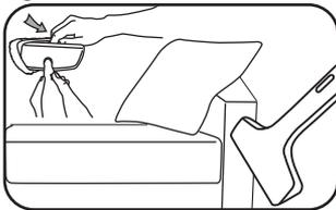
The bed bug / fabric tool with cotton cover is ideal for treating bedding, furniture, pillows, and carpet areas around bed posts and base boards. Start by installing the supplied cotton cover on the clothes - fabric / smooth surface tool. Apply light consistent pressure and slowly pass it along the surface (1" per second) to insure the area being treated has a chance to come to full temperature killing pests and their eggs. (Fig.1)
