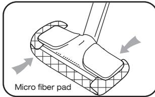
The floor head smooth surface is ideal for stone, tile, vinyl and wood floors along with cleaning washable walls and any hard surface. It can also be used to sanitize, deodorize, kill allergens, bed bugs and dust mites. Attach the micro fiber pad to allow the floor cleaning head to glide when using on carpet. (Fig.3)
