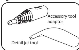
The accessory tool adaptor or the detail jet tool can be used on their own. These tools are great for cracks and crevices. Make sure to concentrate the steam directly on the area to be treated with as minimal distance as possible. The steam will condense and cool off and will not kill pests and their eggs if the jet tip is not directly on the surface being treated.
