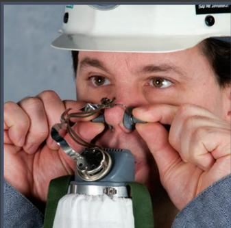
**10** Pull the pads of the noseclip apart and position pads over the nostrils.
