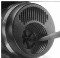
2. Thread the motor-blower coupling nut into the facepiece until resistance is encountered. Continue tightening the coupling nut an additional 60 degrees (the distance of two notches on the coupling nut) into the facepiece.
