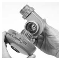
6. Line up the key on the battery cable plug with the slot in the female connector on motor-blower.
