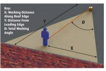
For example, if the anchorage connector is 6' from the leading edge (Y), the working distance (X) is 8' in each direction from the perpendicular, which translates to a 53° working angle.
