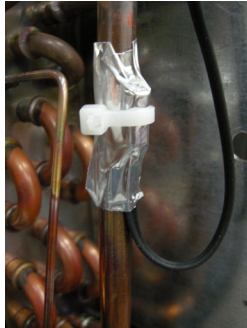
Thermistor attached to the refrigerant line.
