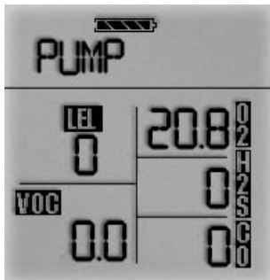
Figure 3-4a. Pump Alarm on the Display
