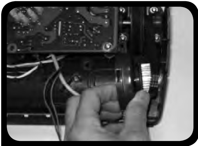
9. Remove clutch assembly - Slide belt off pulley
