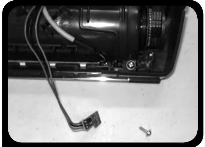
4. Lift straight up on sensor control board, do not lift by wires
