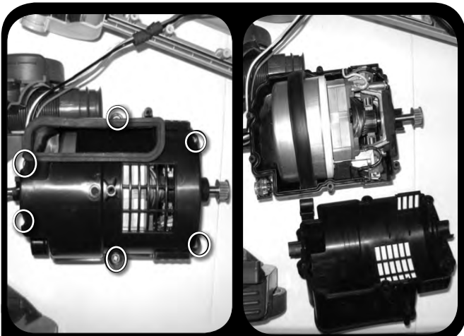
11. Remove upper motor housing - Remove six (6) (M4 x 16mm length) screws
