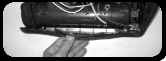
1. Remove rubber bumper - Pull straight up
