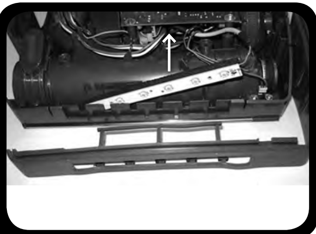
5. Remove LED light - Lift straight up on sensor control board, do not lift by wires
