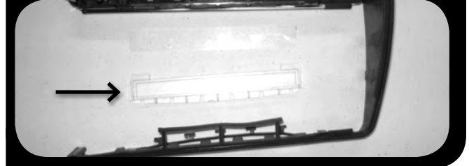
2. Remove lens - Lift up on corner
