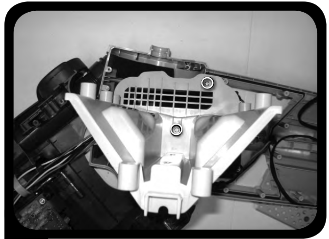
10. Remove air separator - Remove two (2) (M4 x 20mm length) screws
