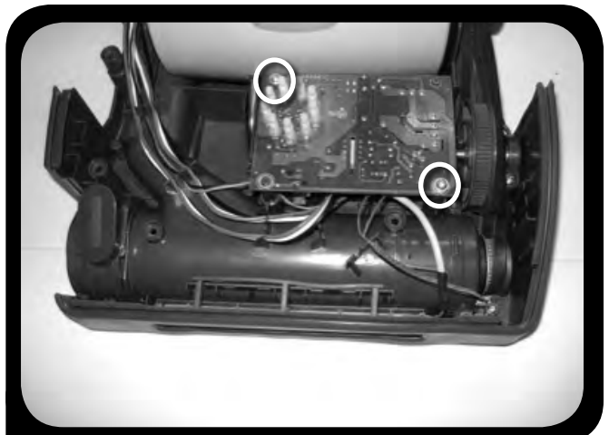
6. Remove printed circuit board - Remove two (2) screws (M4 x 16mm length)
