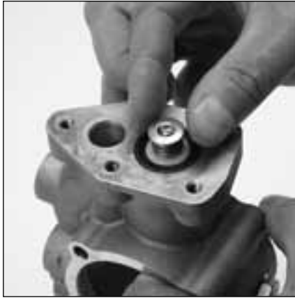
6.20 Install washer (17) with curved surface down on to spring (18).
