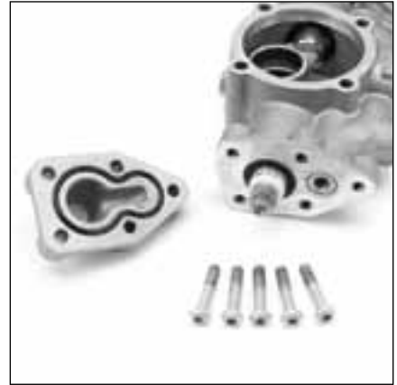
5.10 Remove five (5) M6x30 button head screws (13) holding head cover (14) to crankcase body.
