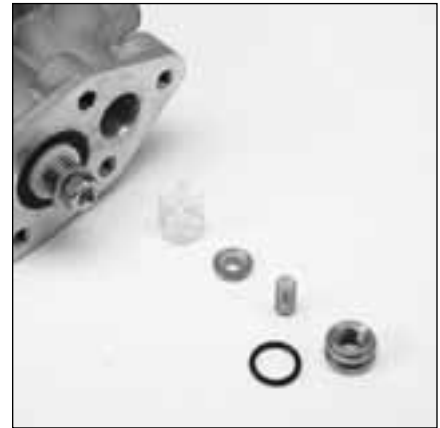
5.13 Separate and inspect retainer (27), spring (26), valve (25), seat (24), and o-ring (23).
