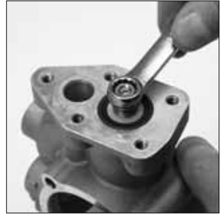
6.21 Apply Loctite®242® to M6 threads on plunger rod. Thread nut (16) onto M6 threads of plunger rod and torque to 25 in-lbs.
