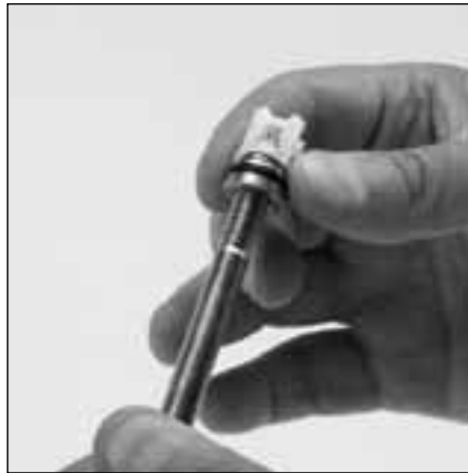
5.12 Thread M8 bolt so it makes contact with valve, continue threading until separation of retainer and seat.
