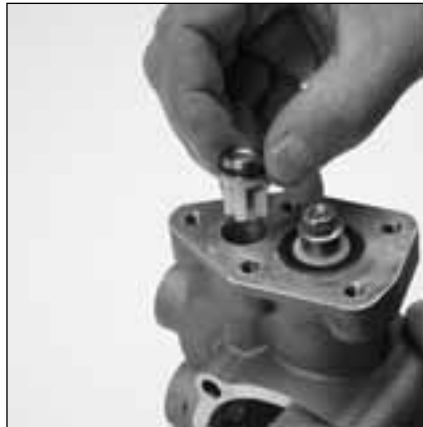
6.14 Press discharge valve assembly (30) into top hole with retainer facing into crankcase body (1) until flush with cylinder head surface.
