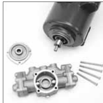
5.3 Separate pump (1) from motor (2) by removing four (4) M6x75 button head screws (4) from bearing cover (5).
