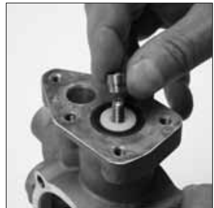
6.18 Install spacer (19) small diameter down into inlet valve (20).
