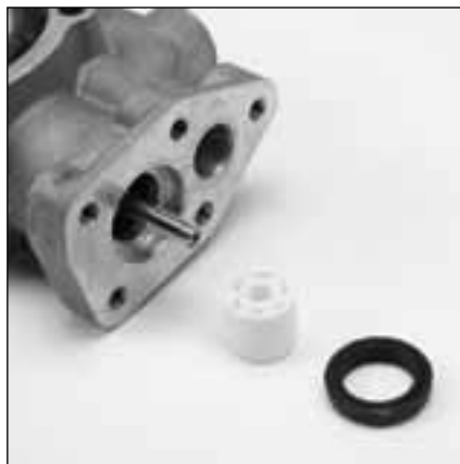
5.15 Remove and inspect ceramic plunger (21) and high pressure seal (22) from crankcase body (1).
