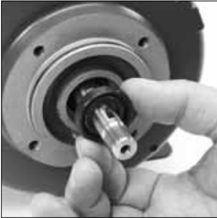
5.8 Remove and inspect shaft seal (10) from motor flange.
