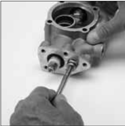
5.11 Remove discharge valve assembly by using M8 threaded bolt.
