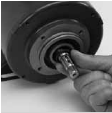
6.1 Lubricate and install slinger o-ring (11) onto motor flange by sliding over motor shaft. Center between shaft seal bore and back of the slinger seal bore.
