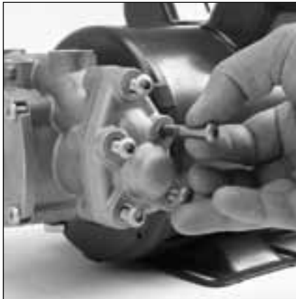
6.23 Position head cover (14) onto crankcase body (1) and hand thread in five (5) M6x30 button head screws (13).
