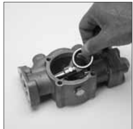
5.16 Remove and inspect connecting rod, plunger rod and wrist pin assembly.
