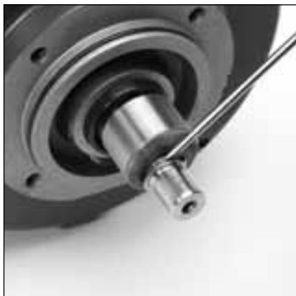
5.5 Remove and inspect retaining ring (7) from motor shaft.
