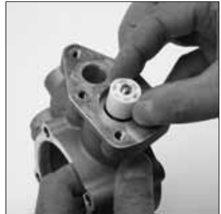
6.15 Install ceramic plunger (21) with larger ID over plunger rod threads. Ceramic plunger can only be installed one way.
