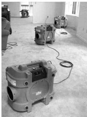
FIGURE 5 Units daisy chained
