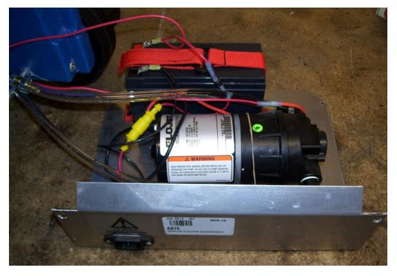
4. Remove the two wire connections from the Battery and cut the wires off close to the connectors. A soldering iron may be needed to remove connectors from battery. Be careful not to damage battery terminals.
