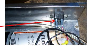
7. From the outside of the base plate, insert the new power receptacle ① through the hole where the old receptacle was. Position the receptacle so the cap is on the right side.
