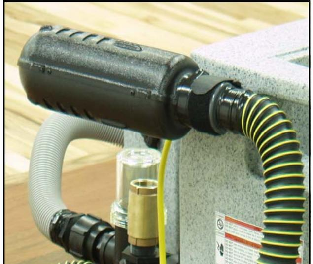
Use the provided velcro loop (power cord strap) to secure temporarily keep the Silencer up from the floor. The hot air from the AR OUT Main hose can cause damage to the flooring materials.
