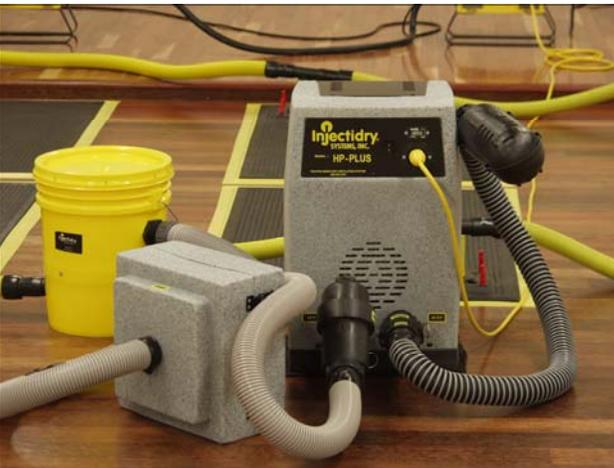
If using an Interceptor HEPA filter, attach the Main Y to the end of it's AIR IN hose and to the panel hose. You may now tape the Vac-It Panels down to the floor (test tape to be used in a hidden location first to prevent finish damage).
