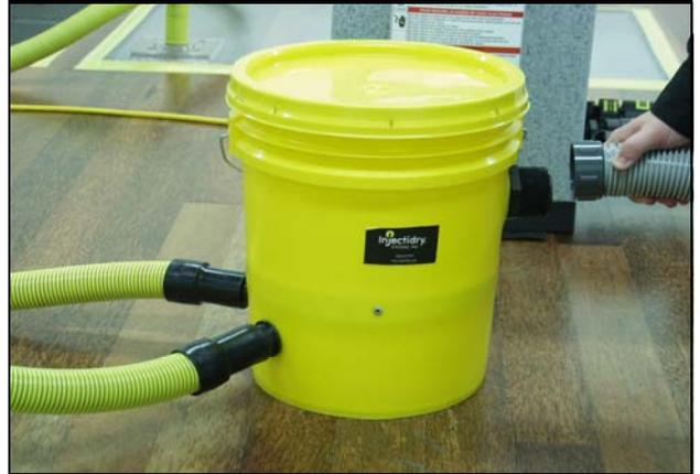
After you have finished extracting, we recommend the use of the WS for the first 24 hours. This helps catch any remaining hidden pockets of moisture that might still be migrating (with the help of the HP unit).
