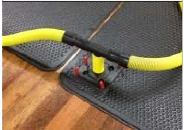
Attach the Panel T's or tubing from manifolds to the main drying lines.
