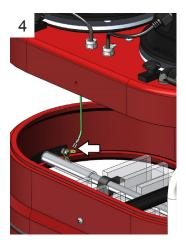
Disconnect the motor deck ground wire from the subsequent assembly via the push-on terminal.
