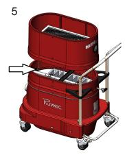
Place the HEPA Maxx module on the machine on top of the HEPA and connect the ground wire.
