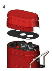
Lift motor shield up from deck to expose motors.
