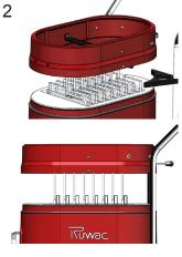
Place in the filter cage housing spacer assembly, making sure to keep the ground wire flat.
