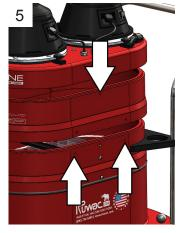
Open up three holes using a 1/2" bit (two holes on filter ring, one hole on HEPA 2.0 ring both sides). 9
