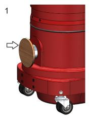
Place the vacuum under pressure by blocking the inlet with a flat and rigid material, and turning on the vacuum.
