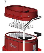
Remove the filter cage housing spacer assembly.
