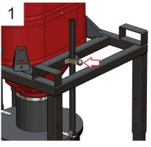
Standing on either side of the machine, grab the ball pin lock and pull it out of the guide.
