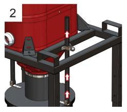
Once ball pin is released, pull up on the guide bar until it locks in the upward position, making sure the ball pin clicks into its designated hole.
