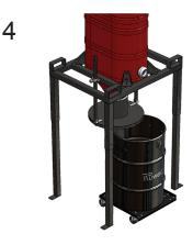
Once both pins and lid are locked in the up position, remove the drum by rolling the caddy unit from under the silo.
