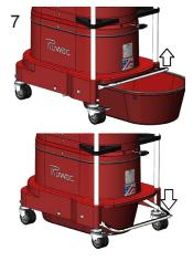
Carefully tip the machine back onto the casters, and replace the dustpan. Lock into position with the footactuated lever.
