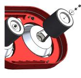
Install the filter and hardware. Tighten standard nut first, then add the locknut to ensure assembly doesn't come loose.
