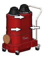
Drill holes into the housing with a 5/16in bit. There are three locations on each side.
