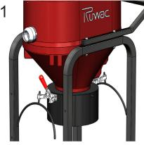
Move each handle into the up position (handle above horizontal position.) This moves the bag clamp away from the valve.
