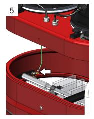
Connect the motor deck ground wire from the subsequent assembly via the push-on terminal.
