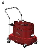
Install the handle bar bracket screws with a 5/32 hex-wrench until the brackets are secure.
