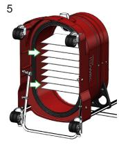
Vacuum off any excess material with another vacuum, making sure not to use any sharp tools that may tear the filter.
