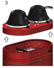
Separate and remove the motor deck from the housing.
