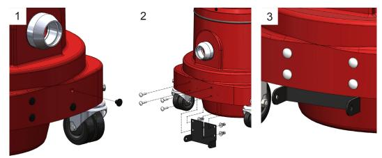
Remove the four plastic plugs from the mounting holes.
