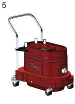
Remove the handle bar bracket screws.
