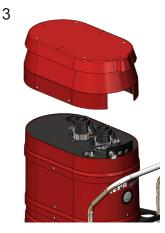
Remove silencer hood from motor deck.
