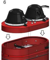
Place the motor deck onto the housing.
