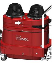
Install all of the hardware which secures the motordeck (both sides) while the vacuum is under pressure. Turn the machine off when done.
