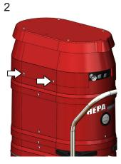
Disconnect hood from motor deck by removing 4 screws.
