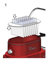
Insert mesh inserts in filter pleats, and seat the filter in the housing.
