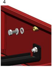
Insert M6 screws and hardware into the back of PEMs.
