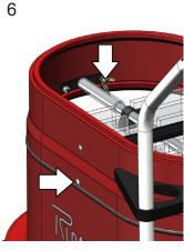
Disconnect the filter housing spacer assembly ground wire from the base via push on terminal. Remove spacer ring screws.
