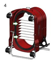
With machine off, knock material off the filter via the manual shaker by moving it in and out rapidly for 10 seconds. Pull up on the dust pan lever to release the dustpan to the floor, and remove the dustpan.
