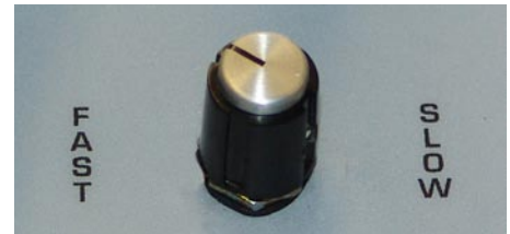
Figure 5: The Hydro-X can move from 1 to 28 feet per minute with the use of the speed control knob.
