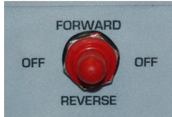
Figure 3: Directional controls feature forward, reverse and off. In the “off” setting the Hydro-X will not move when the movement lever is depressed.
