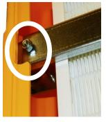
To replace the HEPA filter open the door. You will see 2 filter bars holding the HEPA filter in place. See figure 4 below. These bars are secured with 1/4-20 Nylock nuts, which require a 7/16" wrench or socket to remove them. Remove all 4 filter bar retaining nuts and remove the filter bars as well. Slide the HEPA filter out along the filter guides and remove it from the machine. **ALWAYS TREAT THE USED HEPA FILTER AS HAZMAT AND PROCESS IT ACCORDING TO YOUR ESTABLISHED HAZMAT PROCEDURES.**
