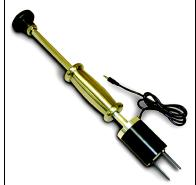
check device supplied with your meter to check the Hammer Electrode and meter (readings should show between 17 and 19%).
