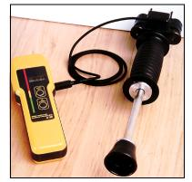
When the Hammer Electrode is not in use, keep it in the packing tube to prevent injury to the user and damage to the pins. Inspect all parts of the Hammer Electrode weekly. If the threaded portions of the shaft begin to show any signs of wear or fractures, stop using the product and contact the *Service Department* immediately at the address provided below.
