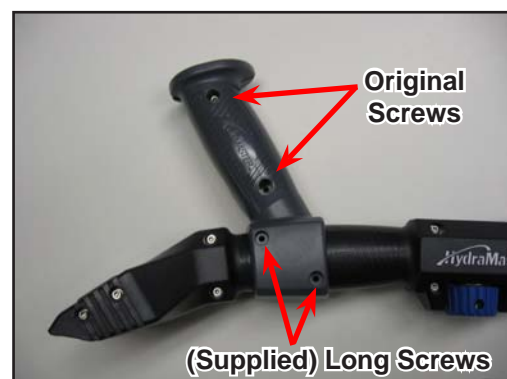
Figure 2-2. Attach Accessory Handle
