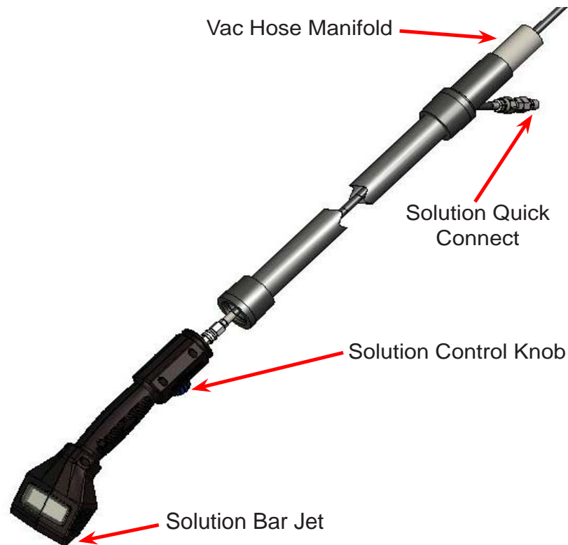
Figure 2-3. Attach Solution Hose and Adjust Water Volume
