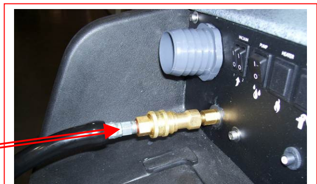
Connect the male end of the HP Solution Hose Assembly to the female solution outlet fitting on the machine. Connect the female end to the cleaning tool.
