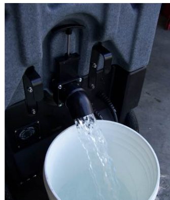
Drain Recovery Tank
