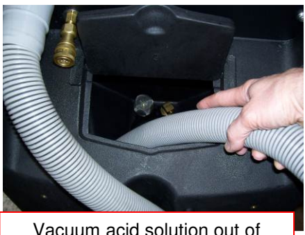
Vacuum acid solution out of Solution Tank
