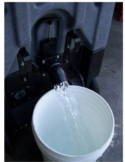
Draining the Recovery Tank
