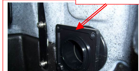
Unless damaged or leaking between tank and flange, the flange fitting does not have to be removed
