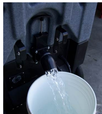
Drain water from Recovery Tank
