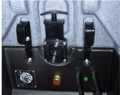
Remove four bolts holding valve assembly to flange fitting
