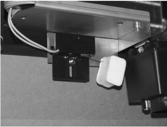
Figure 6: Picture of the float safety switch
