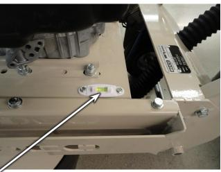
Rock the machine back and forth until the bubble level in centered. This gets the machine close to the proper operating position.
