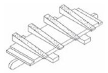
The above in an example of a DYMA-SERT that has hot been rotated after every four hours of use. To get maximum life out of a DYMA-SERT they should be rotated 180° every four hours of use.
