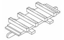
The above in an example of a DYMA-SERT that has been rotated after every four hours of use, as you can see the wear is *even* across all segments.
