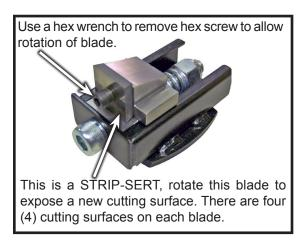
**STRIP-Serts** TM Are carbide-tipped blocks designed to clean floors without grinding into the concrete. The multisided, replaceable tungsten carbides have four edges that can be rotated for maximum use. The carbide Strip-Serts ™ will clean your surface without any damage.
