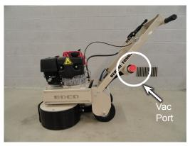
If using a vacuum for dust control attach it to the vacuum port at the rear of the machine which is on the handle as pictured above, securing it with clamps. The port is circled in the above photo. The vacuum port is in the same location on both the gas and electric models.
