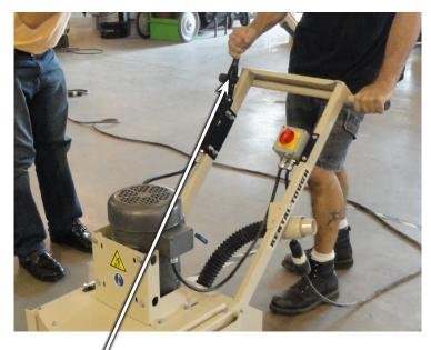
Return level lock to the locked position.
