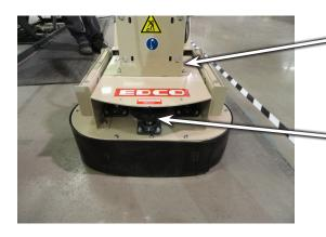
Loosen the four (4) cap screws as in the first step and slide the motor mount all the way forward.
