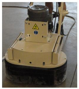
Lean back slightly on the handle to get the tools off of the surface and start the machine. Lower the machine to the surface and do a short touch pass on the concrete.
