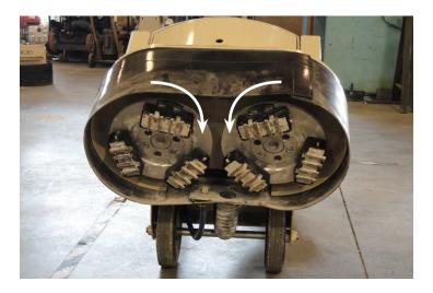
Once all tools are in the proper position return the machine to upright. Remember if you are using tools with PCD's on Stripserts they have a leading edge and must be loaded as such. Also, remember both of the discs turn in direction of arrows.
