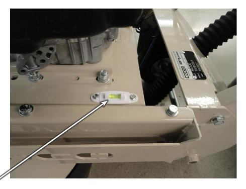
The bubble on the machine will not necessarily be centered once optimum operating position is achieved. It will also float back and forth during grinding. Level on your machine may not be the same as pictured above.
